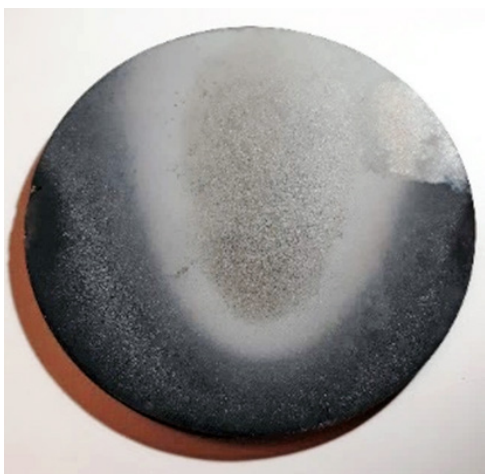
Fig. 19. W3 sample after high temperature oxidation thermal test. Magnification \times 1 . No material sputtering effect occurred
