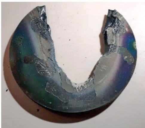
Fig. 18. W2 sample after high temperature oxidation thermal test (failed). Critical material sputtering process occurred. The specimen was destroyed. Magnification \times 1
