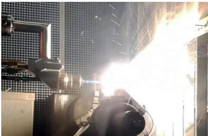
Fig. 1. Thermal test of Nb sample without coating
