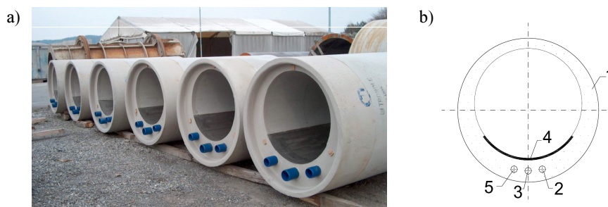
Fig. 3. Heat exchanger integrated in concrete sewage pipe: a) heat exchanger before installation, b) cross-section of heat exchanger; 1 - concrete pipe, 2 - cold water supply to the heat exchanger, 3 - bypass, 4 - heat exchanger, 5 - output of the heated water from the heat exchanger [5]
