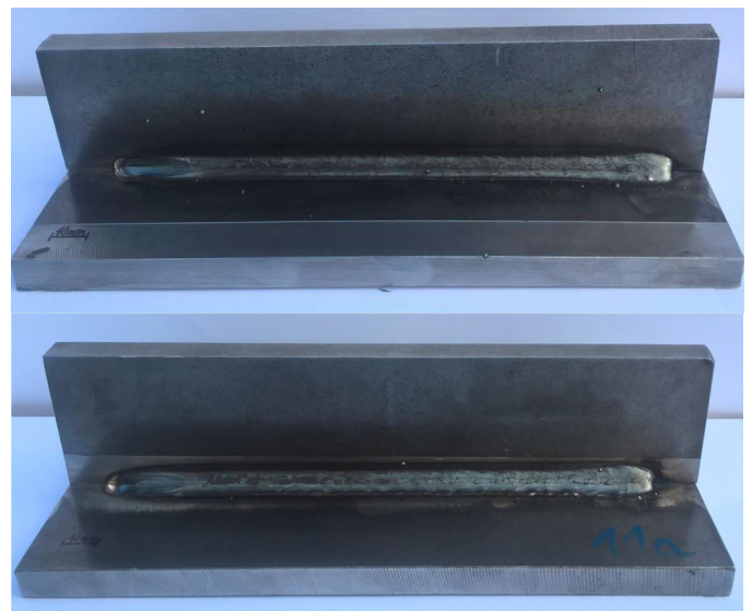
Fig. 5. T-joint welded double-sided welding technique LA
