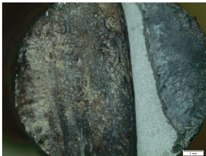
Fig.3. The cross-section view of the damaged anchor.
