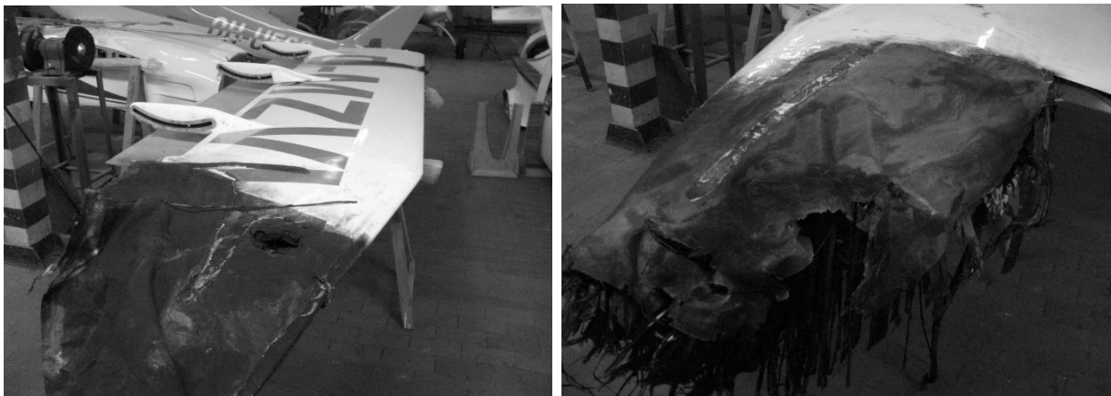
Fig. 1. View of the fragments of the left wing of a UL plane burnt in an aircraft crash involving another UL plane (irreparable)
