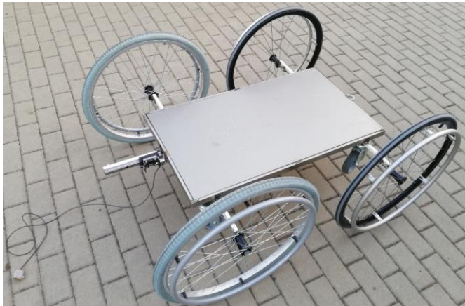
Fig. 3. Research trolley with pneumatic wheels used in wheelchairs
