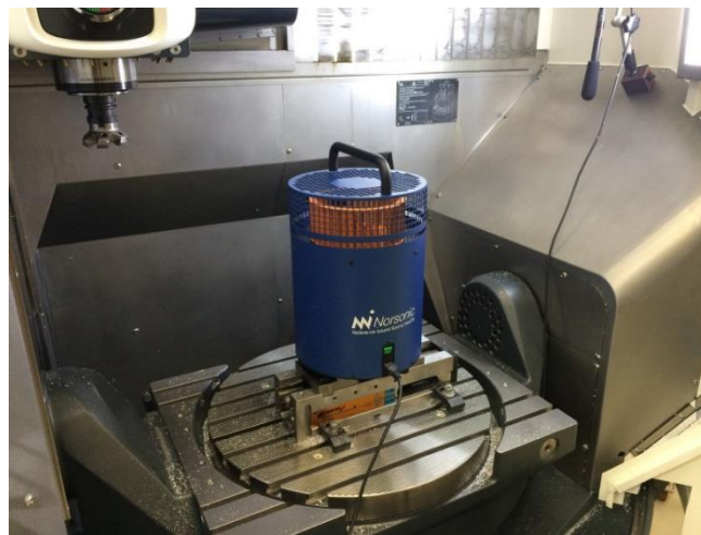
Fig. 3. Noise source placed on the work piece table and inside microphone #64 on the top right side
