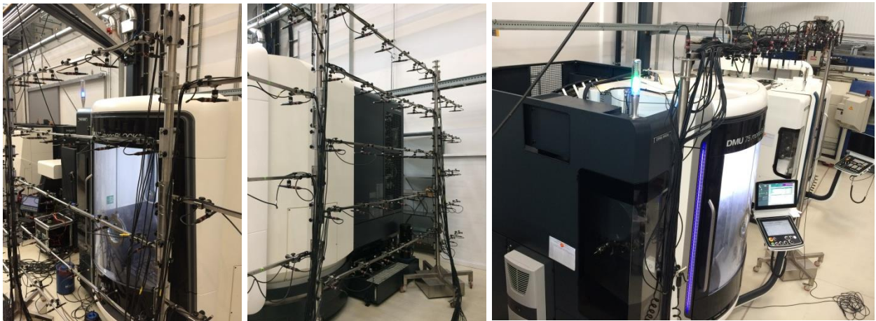
Fig. 1. Vertical microphone grid for measurements of the front machine side (left), of the right machine side (middle) and horizontal microphone traverse for top measurements placed in front of the machine (right)
