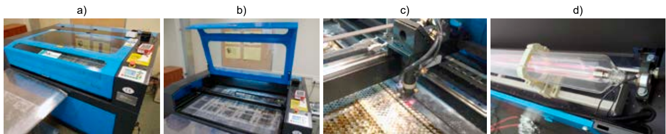
Figure 2. CO 2 laser plotter: a) general view with closed cover, b) inside after lifting the cover, c) laser head with nozzle on slides, and d) laser tube with propylene glycol
