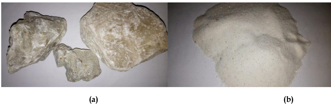
Fig. 2. Azara-Nassarawa barite mineral ore (a) As-received; and (b) Pulverized samples
