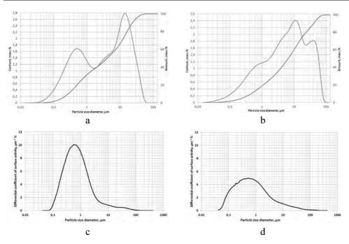
Fig. 2. Particle size distribution (a, b) and differential coefficient of surface activity (c, d) of Roman cement and multicomponent cement
