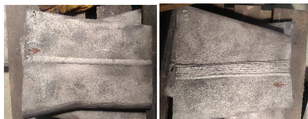
Fig. 3. Test sample with a weld deposit for repairing the crack and narrow defects (left) and for repairing flat defects (right)
