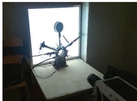
Fig. 1. Test bench with isochoric combustion chamber
