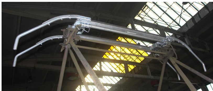
Fig. 11. Testing collector shoe installed on the pantograph
