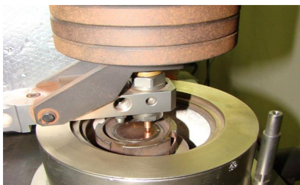
Fig. 3. View on samples during friction testing
