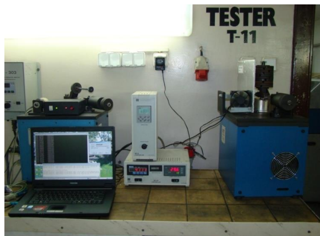
Fig. 1. The T-11 tribological test stand
