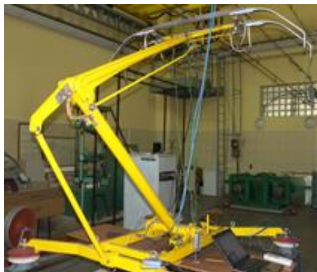
Fig. 4. Test stand for testing of current collectors
