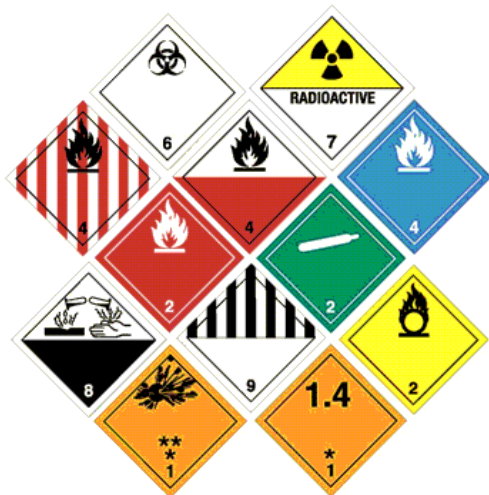
Figure 2. Appropriate labels indicating the hazard (Flammable, toxic, Corrosive etc.) are also pasted over the package. The label must be water resistant such that even in case of immersion, it should be readable for at least 3 months. Source: https://www.portsecuritycenter.eu/handling-imd-g-cargo/
