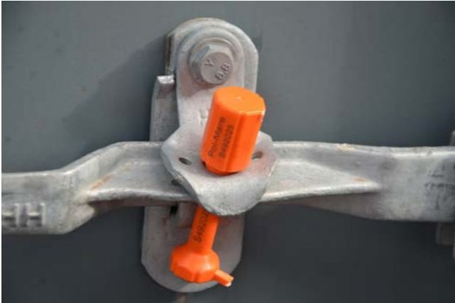
Figure 6. Securing the closure of the container with a bottled seal. Source: Pol-Mare Ltd.
