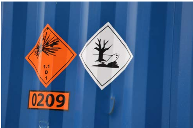
Figure 4. Marking on a container with dangerous goods - Class 1 explosives. Source: Pol-Mare Ltd.
