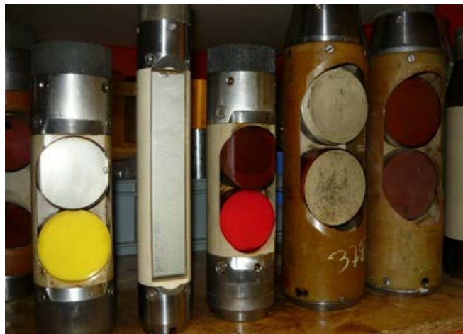
Fig. 7. Different sonar measuring heads with transducers for special survey tasks
