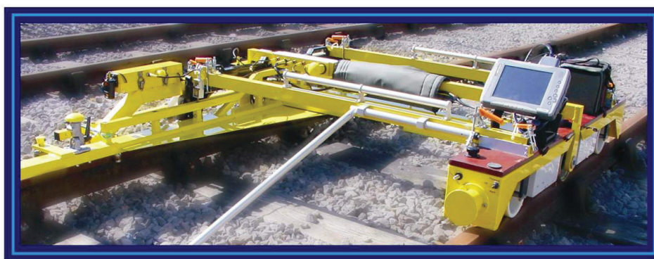
Rys. 4. Track Quality Measurement (TQM) z bazami 3m Hz and 2m VV Certyfikaty: Network Rail CEF12737 and PA05/02253, London Underground PE007/1211
