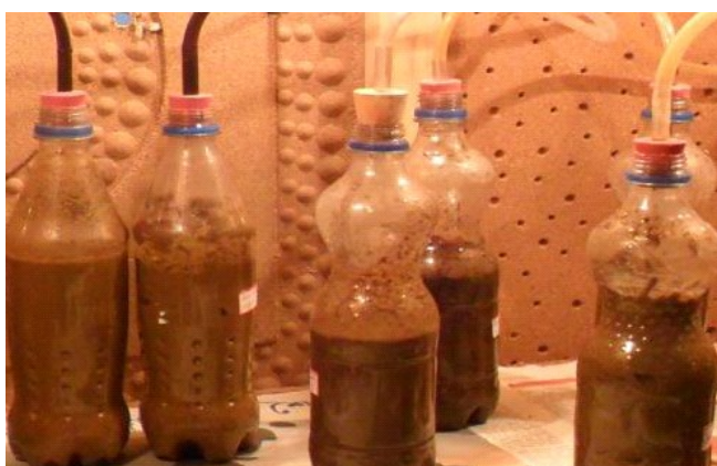
Fig. 1 Bench type photo-bioreactors are arranged in batch mode
