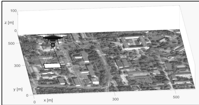
Fig. 2. Illustration of the observation process using a monocular camera installed on UAV.
