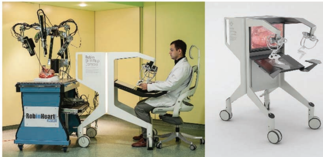
Fig. 8. Robin Heart Tele robot with a control console equipped with motion controller with force feedback
