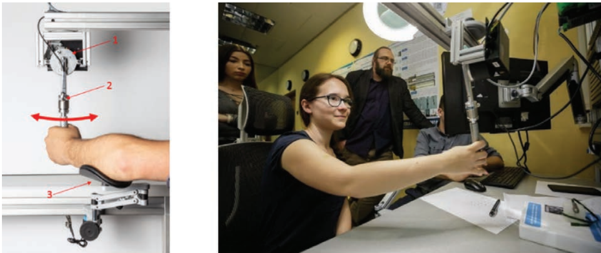
Fig. 4. Measuring stand for verification of force impacts on the operator
