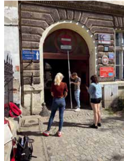
Fig. 6. Measurement of the facade and gate using a staff, inventory in 2022; source: author – Antonio Nevescanin
