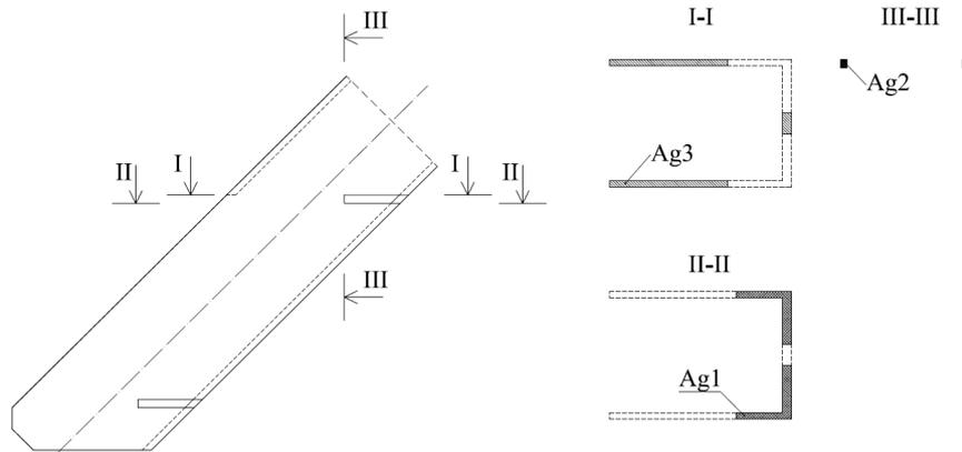
Fig. 5. Tension brace view – top connection
