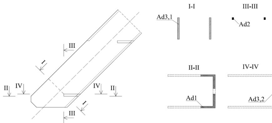
Fig. 6. Tension brace view – bottom connection
