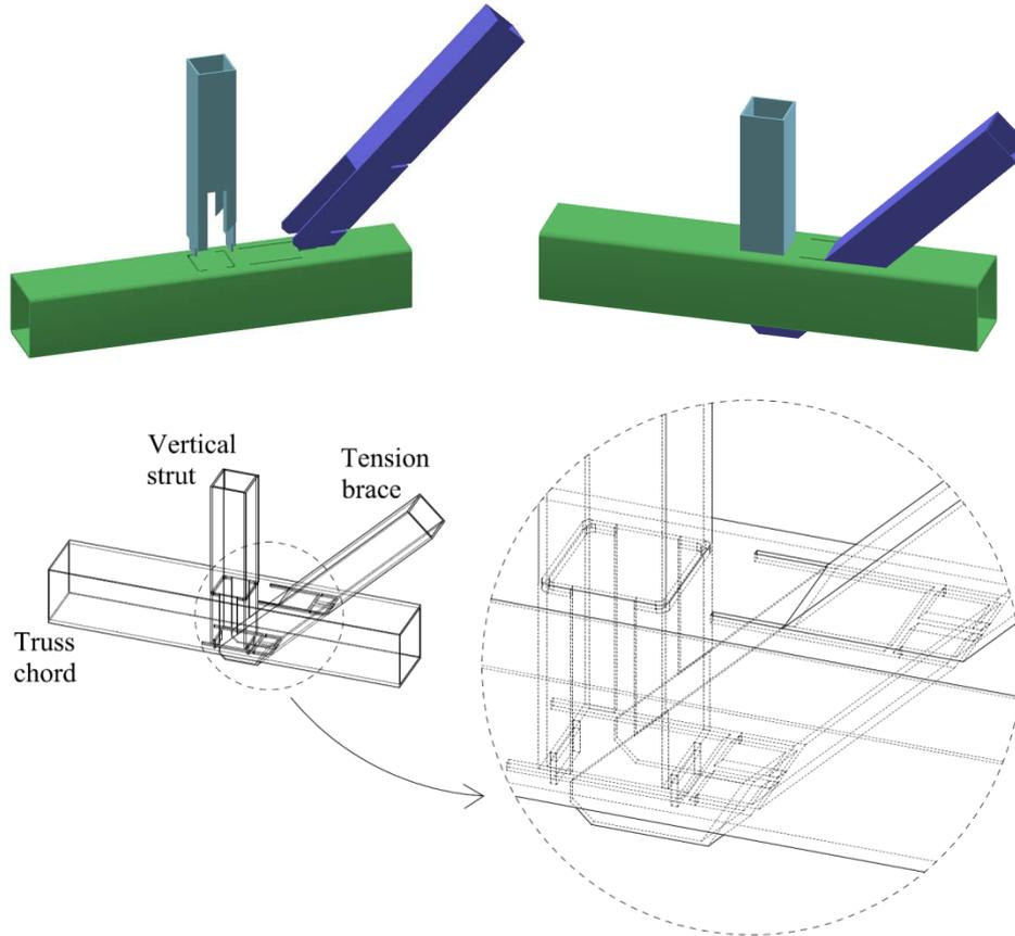
Fig. 3. Concept no II – plug & play N-shape connection, 3D model
