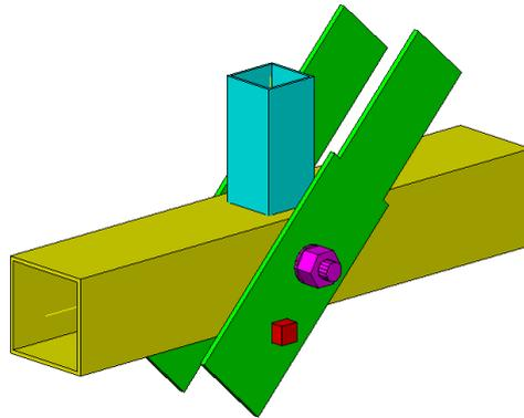
Fig. 1. Plug & play N-shape connection, 3D model [5]
