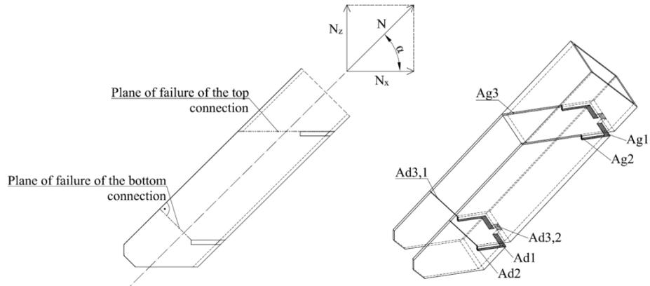
Fig. 4. Tension brace side view and 3D view, where:  $A_{g1}$ ,  $A_{d1}$  – stress area perpendicular to  $N_z$  force,  $A_{g2}$ ,  $A_{d2}$  – stress area perpendicular to  $N_x$  force,  $A_{g3}$  – area of failure of the top connection,  $A_{d3,1}$  – area of failure of the bottom connection (subjected to tension),  $A_{d3,2}$  – area of failure of the bottom connection (subjected to shear and tension)
