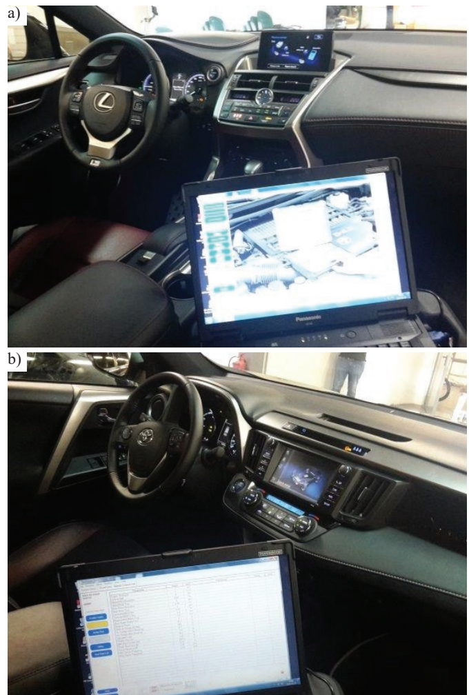
Fig. 1. Vehicle test conditions using on-board diagnostic system reader designed for analysis of vehicles with hybrid drive systems
