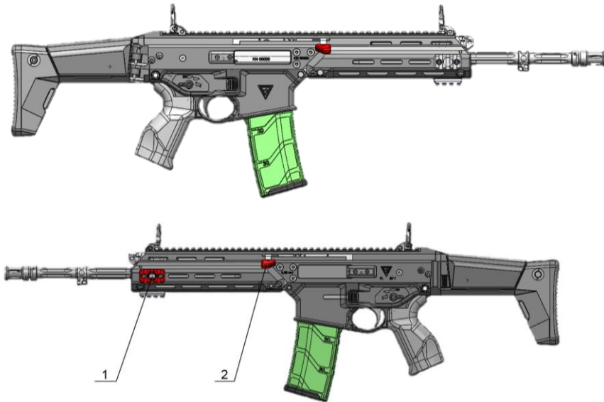
Fig. 3. Modifications committed to the MSBS Grot calibre 5.56 mm standard (basic) assault rifle, version A1: right-hand view (top image); left-hand view (bottom image): 1 – side rail with a carrying sling QD port; 2 – heavy-duty universal cover of the charging handle, fits RH and LH sides
