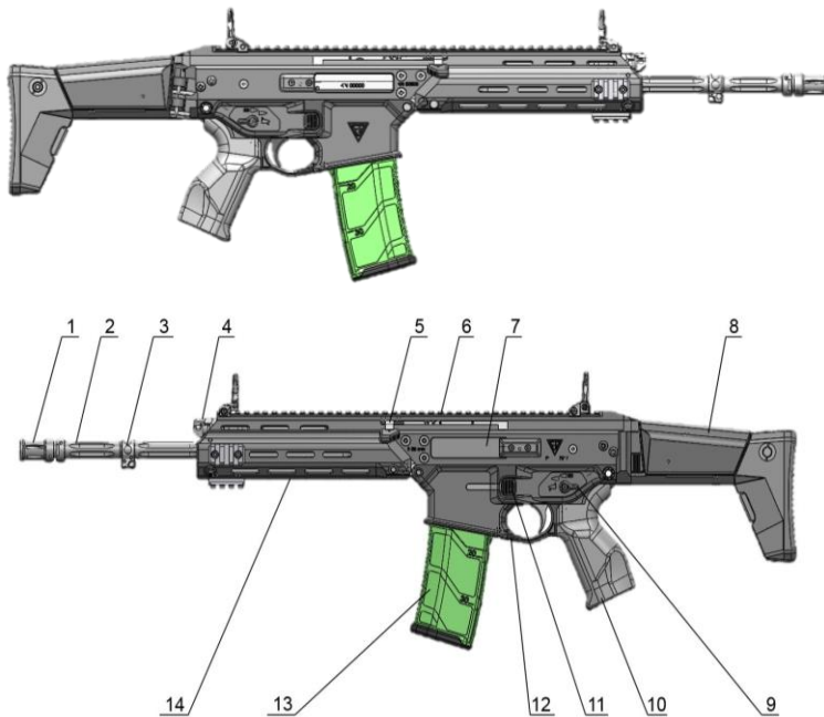
Fig. 2. MSBS Grot calibre 5.56 mm standard (basic) assault rifle, version A0: right-hand view (top image); left-hand view (bottom image): 1 – flash suppressor; 2 – interchangeable barrel; 3 – knife/bayonet mount; 4 – two-position gas regulator; 5 – charging handle, two-sided; 6 – upper receiver w/full-length Picatinny rail (STANAG 4694); 7 – two-sided ejection port with spent case ejection side switchover capability; 8 – telescoping buttstock (5-position), folding away to the right-hand side and complete with an adjustable cheek pad; 9 – two-sided safety/fire mode selector lever; 10 – interchangeable AR15/M16 style pistol grip (imported); 11 – two-sided magazine catch; 12 – two-sided bolt catch; 13 – AR15/M16 style magazine; 14 – handguard with mounting rails (MOE) to accommodate, for example, a front grip, a flashlight, or a 40 mm under barrel grenade launcher
