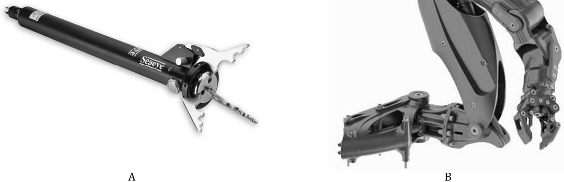
Fig. 3 Manipulators in underwater vehicles. A – GripStick manufactured by Saab SeaEye with a single function [12.e], B – 7-function M700 manufactured by TitanRob [12.f].
