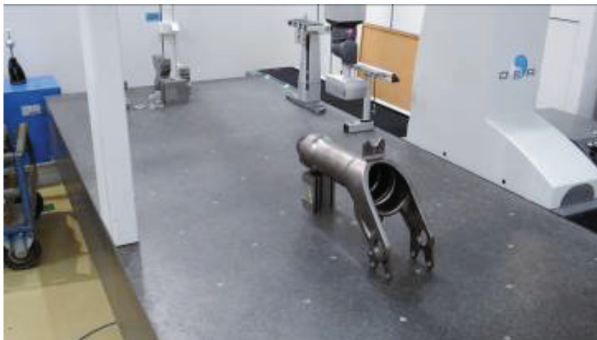
Fig. 5. The measurement taken on the Coordinate Measure Machine equipped with a laser head
