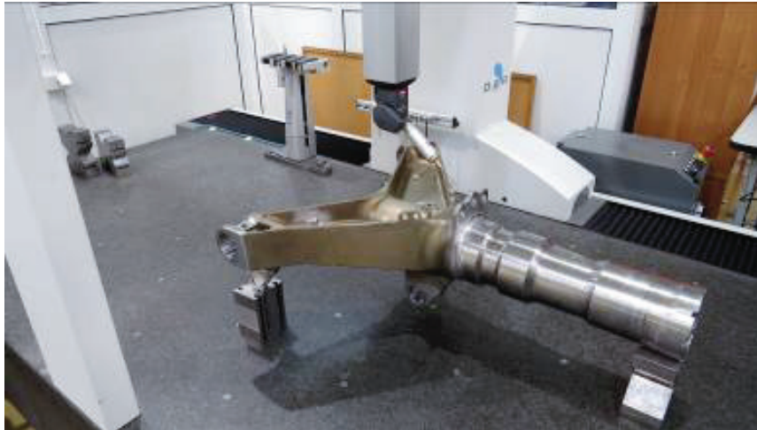
Fig. 4. Taking measurements on the Coordinate Measure Machine
