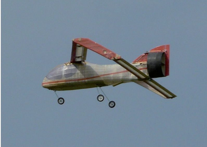
Fig. 9. Final configuration of the model in scale 0.12, equipped with tubular rudder [C. Galiński, 2013]
