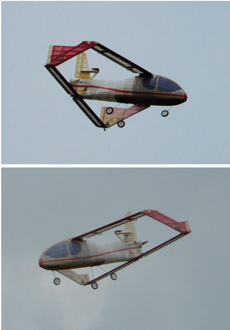
Fig. 7. Experiment showing marginal effect of the area of wingtip plates on lateral-directional stability [C. Galiński, 2013]
