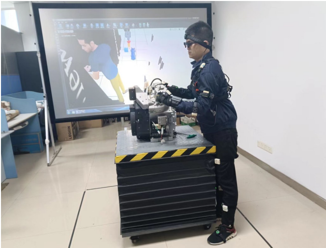
Fig. 10. The virtual–real maintainability test
