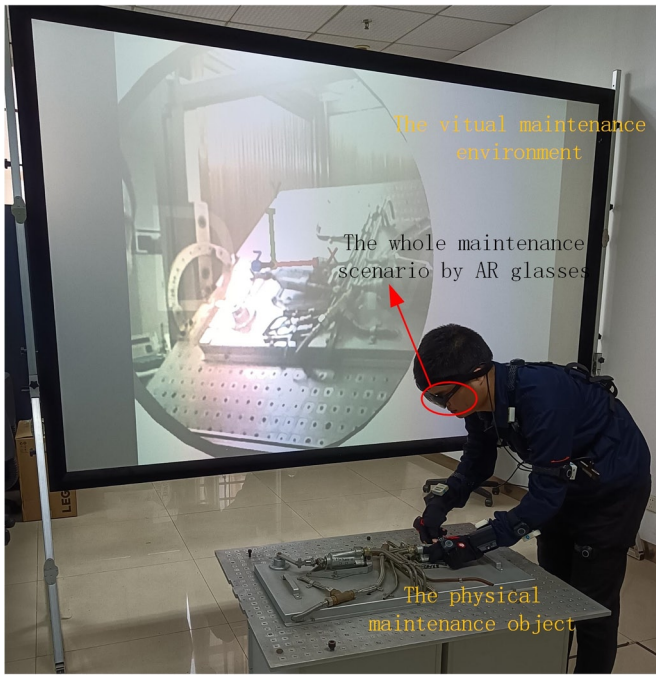
Fig. 3. Schematic of virtual reality integration
