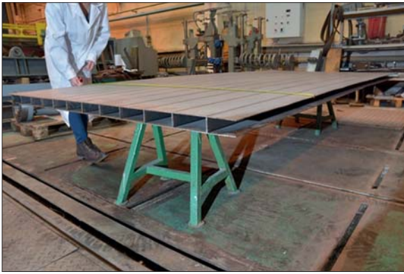
Fig. 1. a) Panel type I-core and b) potential configuration of stiffeners
