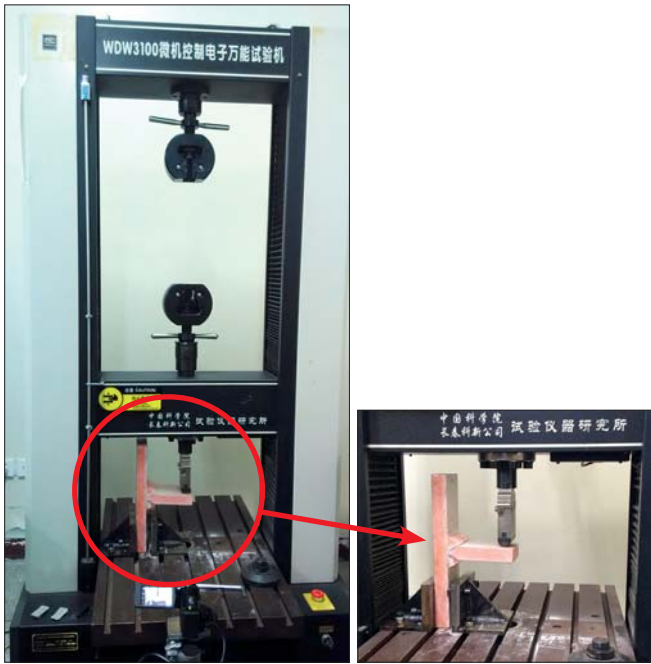
Fig. 6. Mechanical test for the T-type connection specimens
