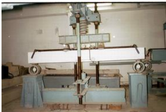
Fig. 4. The testing equipment of beams on long-term loading
