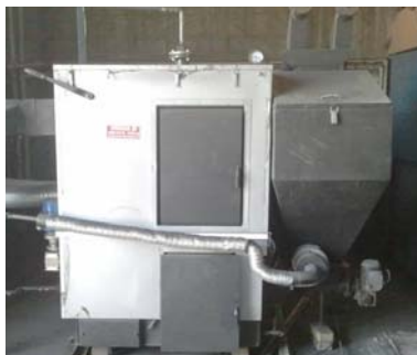
Fig. 1. Prototype of the experimental coal-fired installation built within the scope of the project
