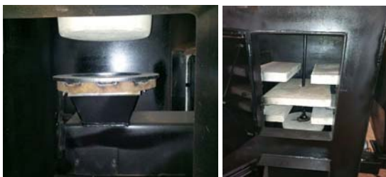
Fig. 2. Furnace interior with the dephlegmator
