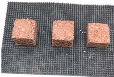
Fig. 4. Samples of ceramic material obtained on the bases of the lightweight aggregate R2, in a dried state
