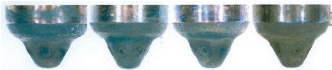
Fig. 3. Photographs of injector tips from FORD Duratorq 2.0 TDCi after test No. 1
