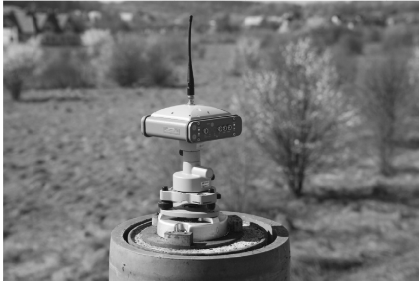
Fig. 3. Topcon HiperPro receiver on GDF21K tribrach – point „0”.
