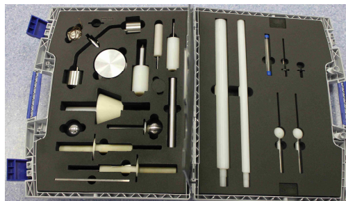
Fig. 4. Access samples for active components used in the laboratory and produced by ITeE – PIB
