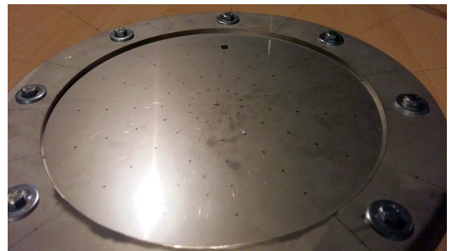
Fig. 1. The investigated circular plate, mounting screws and steel ring.
