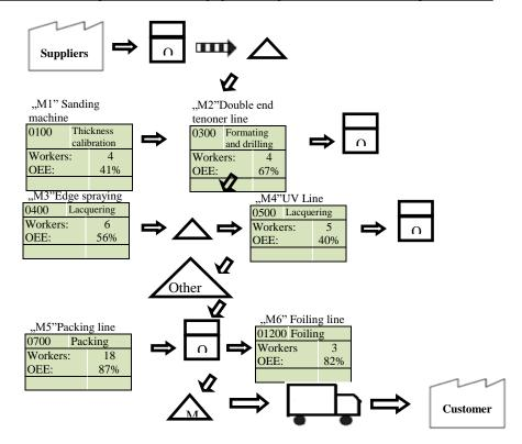
Fig. 3 Simplified diagram of the manufacturing process of cabinet furniture
