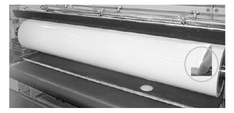
Fig. 6 Roller coater armed with polyurethane shaft (Szwedzka, 2014)
