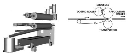
Fig. 5 Roller applicators scheme and way of the lacquer application process
