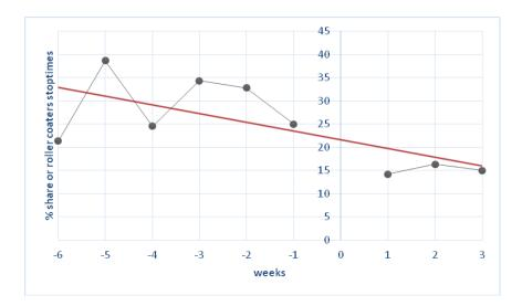
Fig. 8 The percentage of roller coater failures before and after described change
