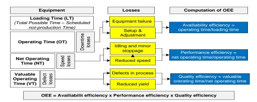
Fig. 1 Computation of OEE (for individual equipment) (Nakajima, 1988)
