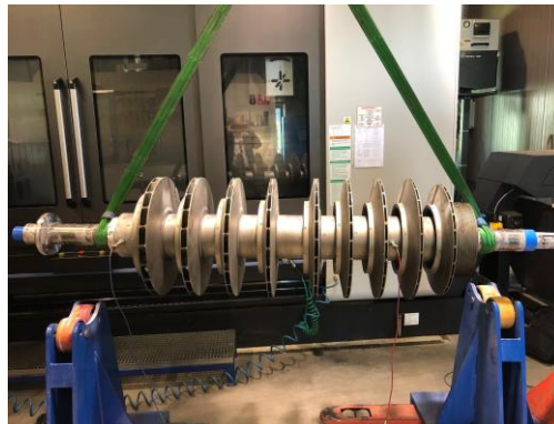
Figure 3. Free-hanging rotor of the compressor during natural vibration measurements for numerical model tuning
