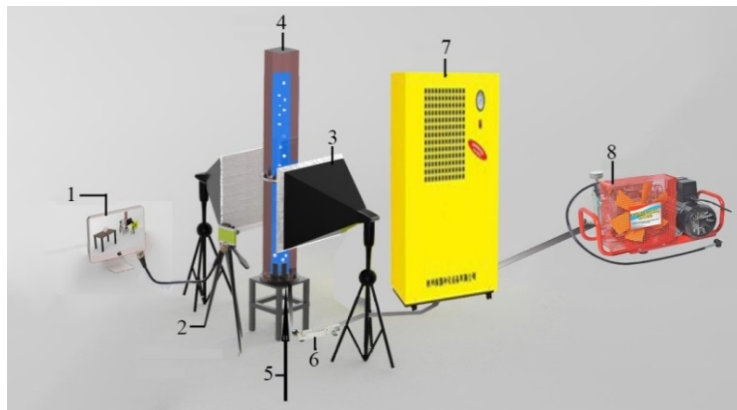
1-computer; 2-high speed camera recorder; 3-LED lamp; 4-simple flotation column; 5-bubbler; 6-gas mass flow meter; 7-flotation column console; 8-air compressor
