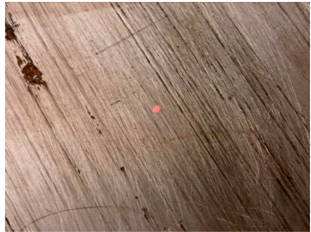
Fig. 5. Crystallizer's desk surface detail with laser dot from laser distance sensor
