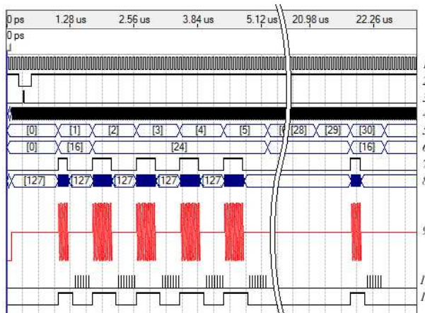
Fig. 6. Simulation of device operation: 1 – 50 MHz clock pulses; 2 – start pulse; 3 – sync pulse; 4 – 250 MHz clock pulses; 5 – memory address bus; 6 – memory address bus; 7 – DDS synthesizer enable pulses; 8 – data bus on DAC; 9 – simulated analog signal; 10 – synchronous detector control pulses; 11 – gating pulses.
