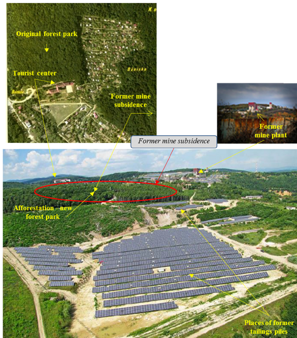
Fig. 8. Mine subsidence and surrounding (Košice-Bankov) after reclamation; panoramic view: summer 2016. Solar collectors in the places of the former tailings piles; afforestation (in the background) in the place of the former mine subsidence
