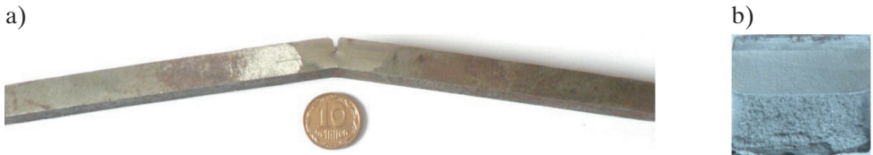
Fig. 2. General view of the sample (a) and the area of its deformed surface (b) after the experiment of researching the conditions of continually operated drill pipes failure
