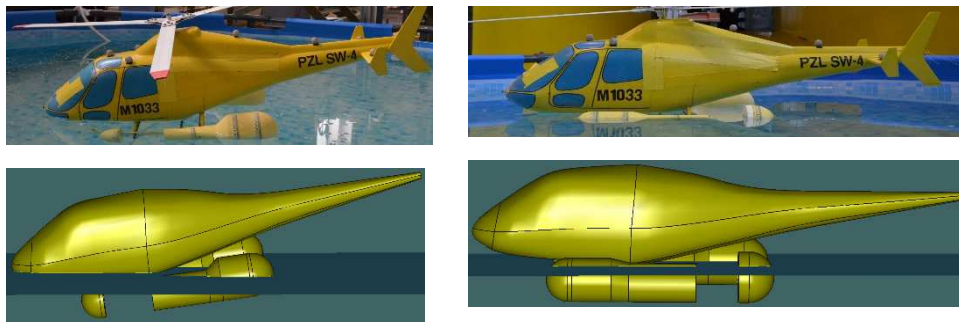
Fig. 6. Computational and model scale experimental verification of the flotation system design
