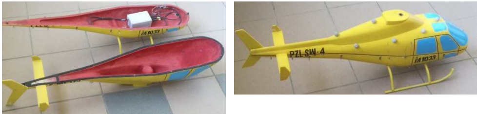
Fig. 9. Model fuselage – dismantled and assembled
