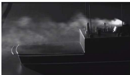
Fig. 4. Experimental validation of the airwake evaluation: wind tunnel model and comparison of computed and measured velocity field (red – CFD, blue – experiment)
