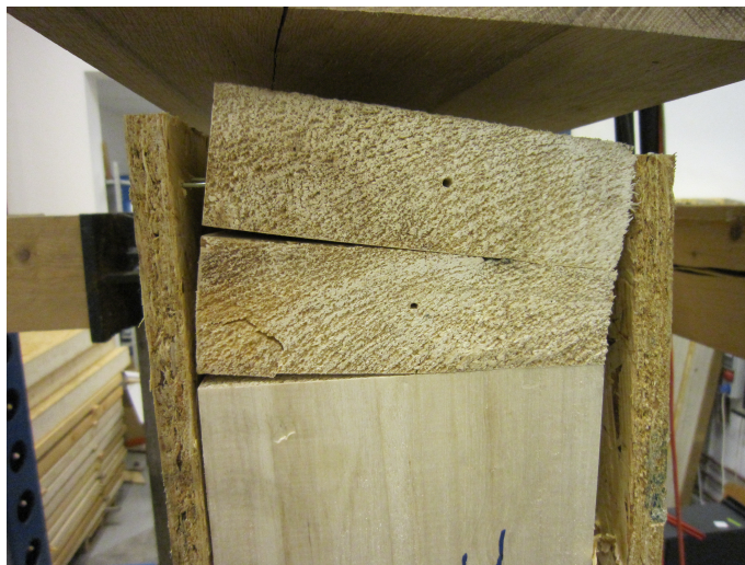
Fig. 5. Deformation of the upper stud
