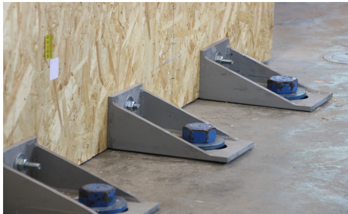
Fig. 3. Fastening to the strong floor
