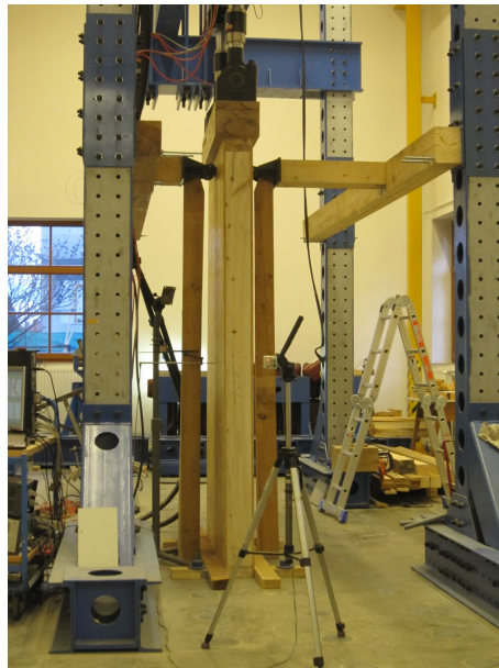
Fig. 2. Compression test measuring position
