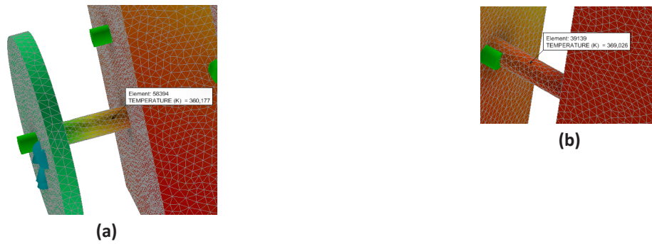
Fig. 4. Satellite temperature in steady state condition: (a) Temperature gradient in antenna positioning mechanism; (b) Temperature gradient in solar panel positioning mechanism
