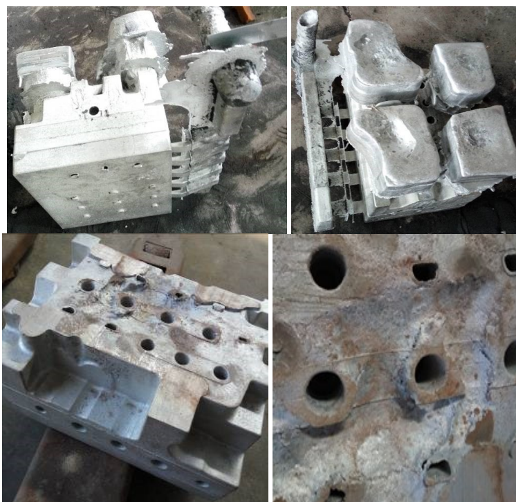
Fig. 15. Casting of single side gating system
