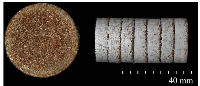
Fig. 1. An example of sample shape (diameter 38 mm) made by extrusion method of aluminum powder with the addition of 2% iron powder at 400°C, and a stack of samples for extruding bars (right picture)
