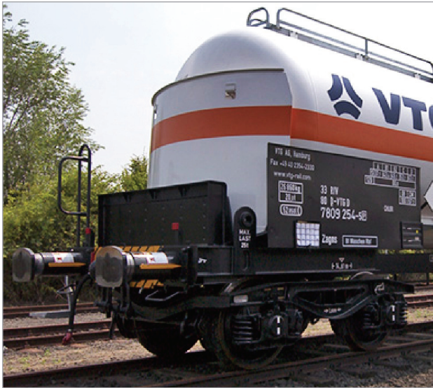
Fig. 5. A tank headstock protective shield and a grip supporting rescue activities [5]
