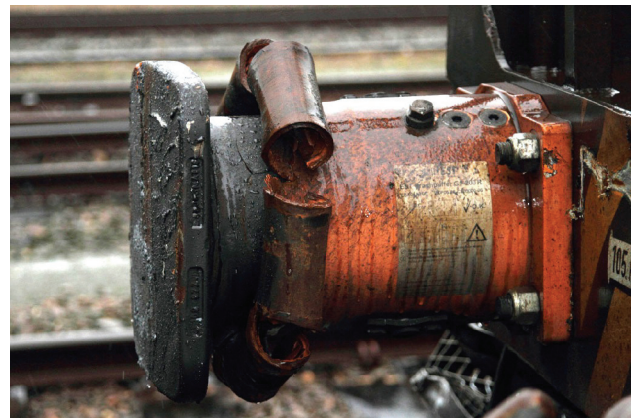
Fig. 2. A buffer absorbing impact energy after plastic deformation of the casing [7]
