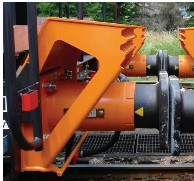
Fig. 4. An EST AC04 anti-climbing module and a deformed EST G2 buffer absorbing impact energy [6]
