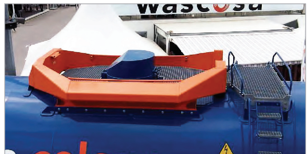
Fig. 7. A UE01 module protecting tank filling valves in the event of tipping over [1]
