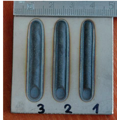
Fig. 4. A view of single stringer beads produced by defocused disk laser beam with a diameter of 6.8 mm on the substrate of stainless steel (bead width in a range of 6-6.5 mm)
