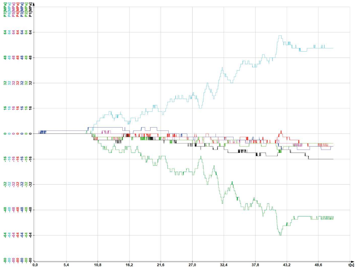
Fig. 12. Downward ride of the elevator car at 4 m/s, with no load [7]
