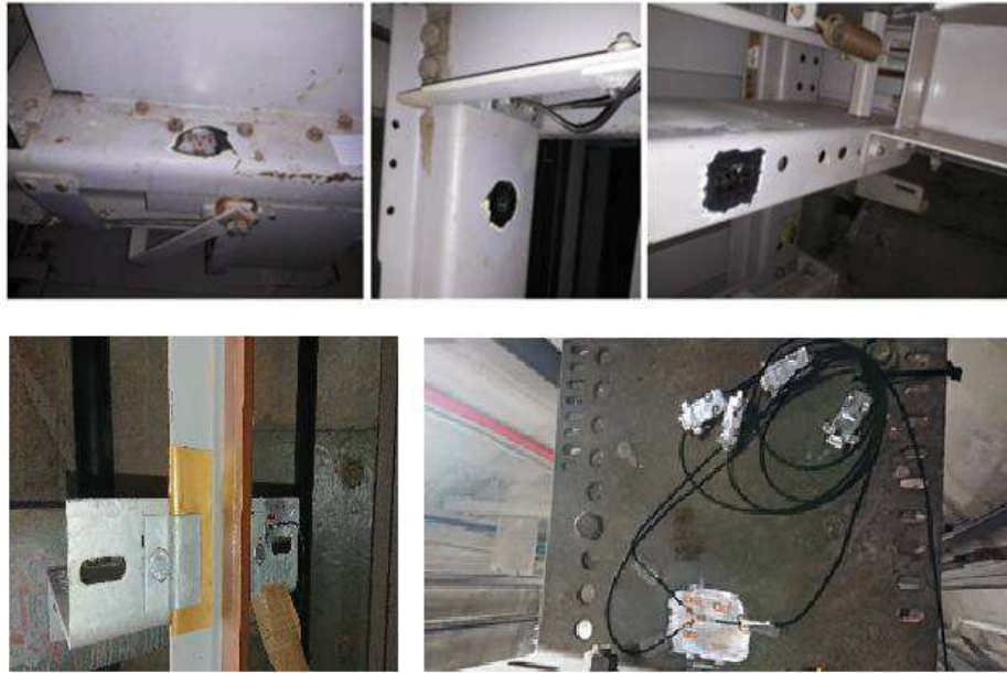
Fig. 11. Strain gauges attached to the selected points on the car frame and east-end supporting beam [3]
